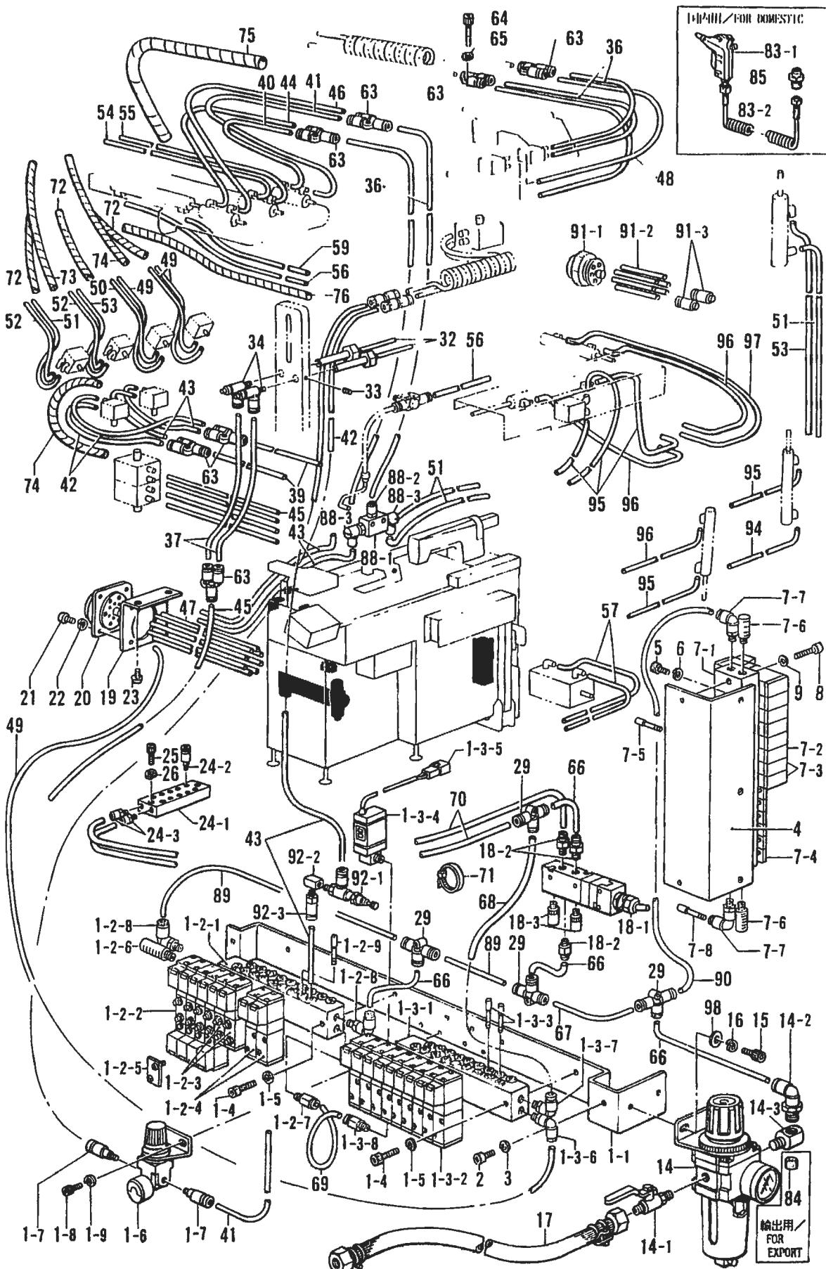
八. エア圧機部/Air pressure mechanism/Luftdruck/
