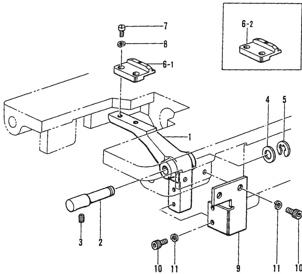
D. 糸切レ感知関係/Thread breakage detector mechanism/Fadenbruchfühler/
