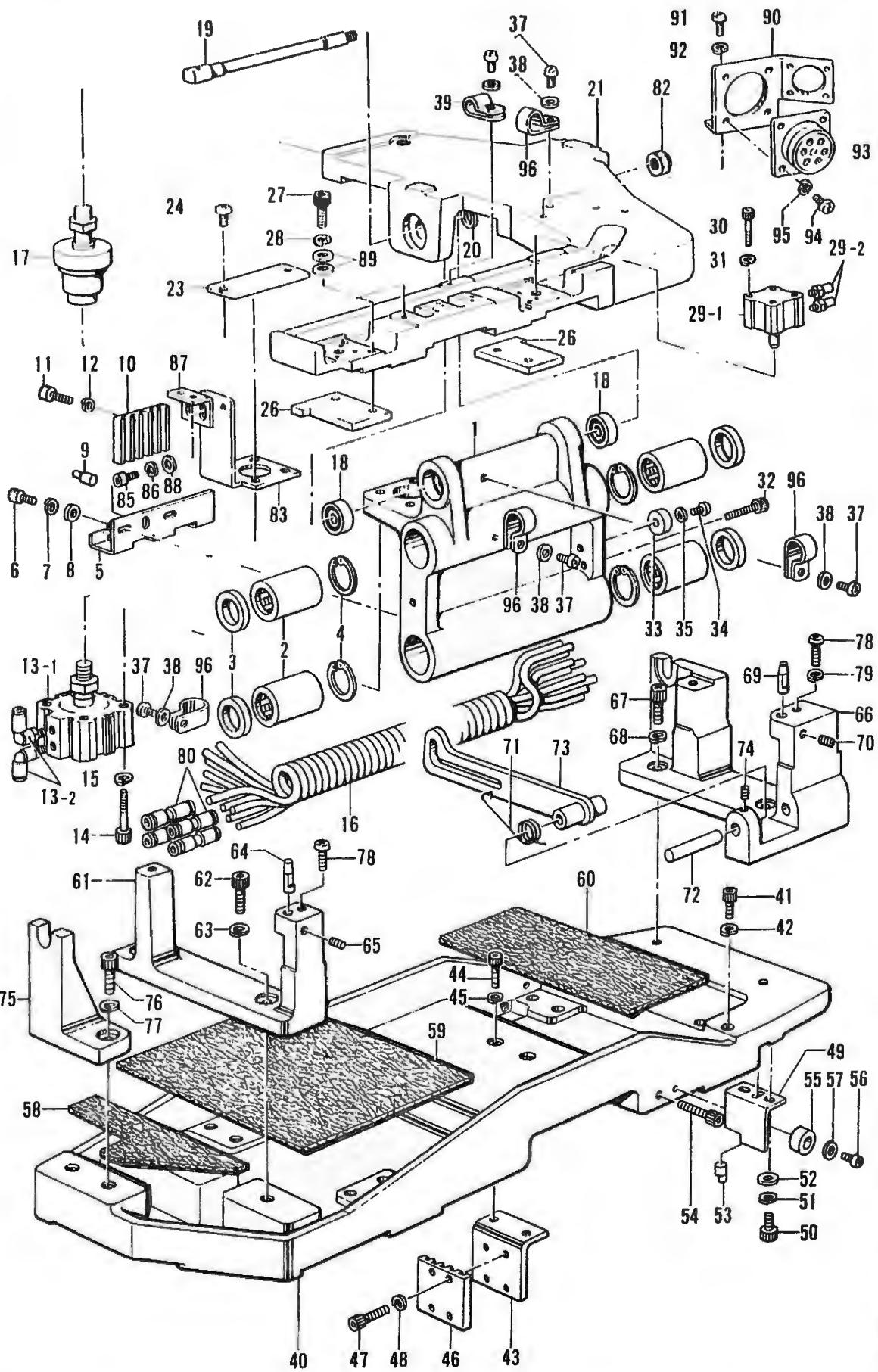
U. 駆動側・送り関係/Drive, feed mechanism/Transporvorrichtung/
