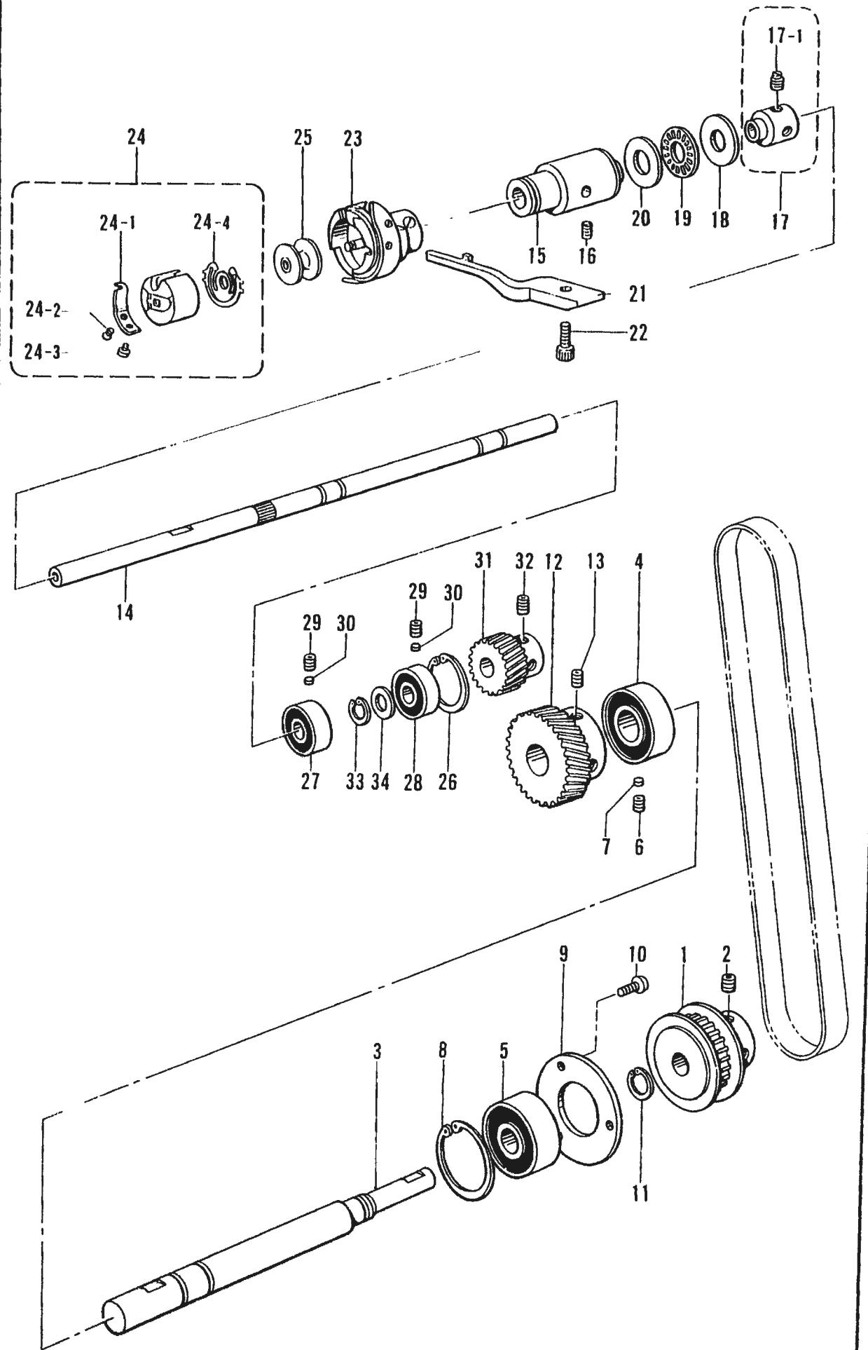
F. カマ関係/Rotary hook mechanism/Greifervorrichtung/
