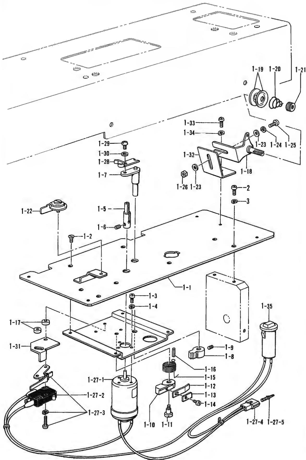
W. 素巻関係/Bobbin winder mechanism/Spuler/
